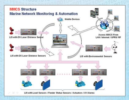
Zalda BIM is one of many applications built upon Zalda's mature MMCS network monitoring – automation platform. It is supported by MMCS multiplex information systems and integrates seamlessly with other MMCS applications such as BSM berthing status monitoring, MLM mooring load monitoring, MEM marine environment monitoring and ACM mooring line release automation systems.
